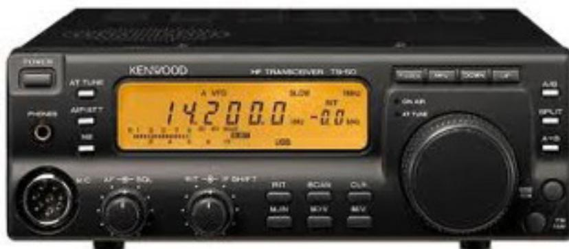
Typical HF SSB Transceiver
